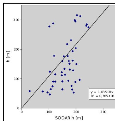
Figure 46. The relationship between stable mixing height calculated from models no. 6 and measured by sodar
