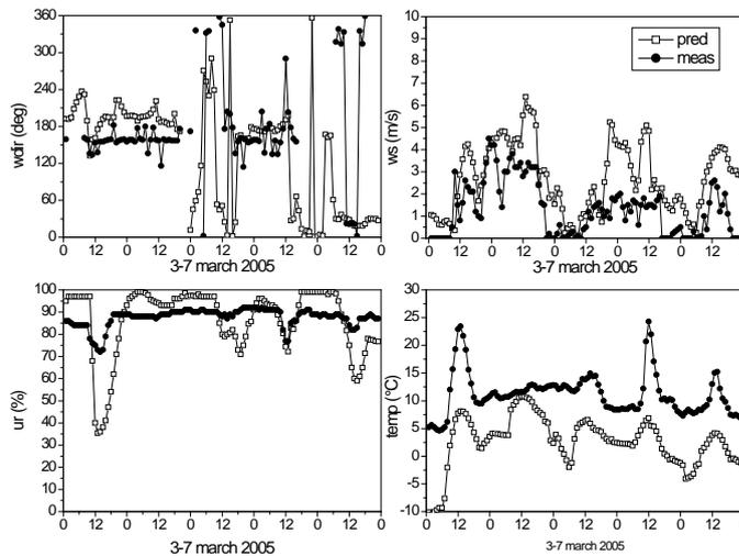
Figure 4. Temporal variation of near surface wind speed (ws) (m s<sup>-1</sup>), wind direction (wdir) (deg), temperature (temp) (°C) and humidity (ur)
