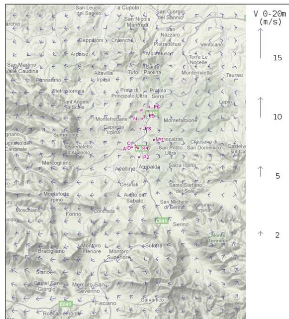
Figure 3. Horizontal wind vectors at ground as simulated by the meteorological models at 8:00 UTC on 3 March 2005. Squares indicate the positions of industrial plants, P1-P6 indicate the position of monitoring samples during the whole field campaign.
