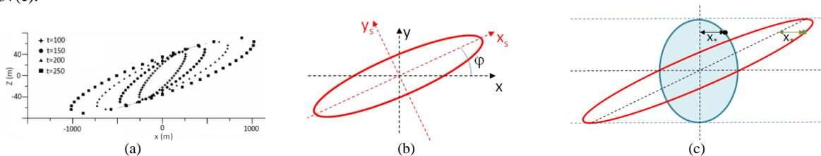
Figure 37: Shear effects on puffs. Puff evolution in pure shear (a). Absolute and shear coordinates definition (b). Coordinate transformation taking shear into account (c).
