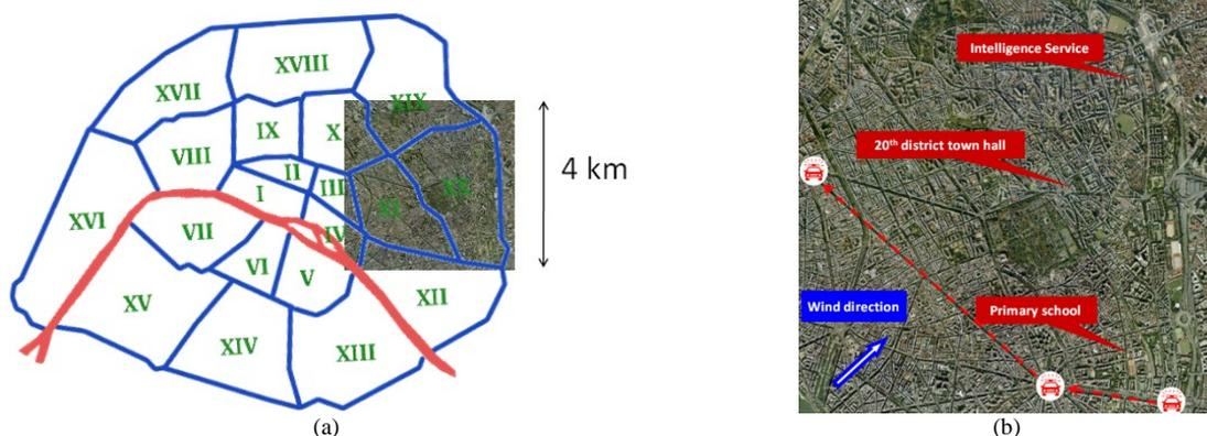
Figure 41 : Overview of the application case of SIRANERISK model on a toxic release from a moving vehicle in East Paris. (a): district situation. (b): Top view: Red arrows show source trajectory and blue arrow shows wind direction.
