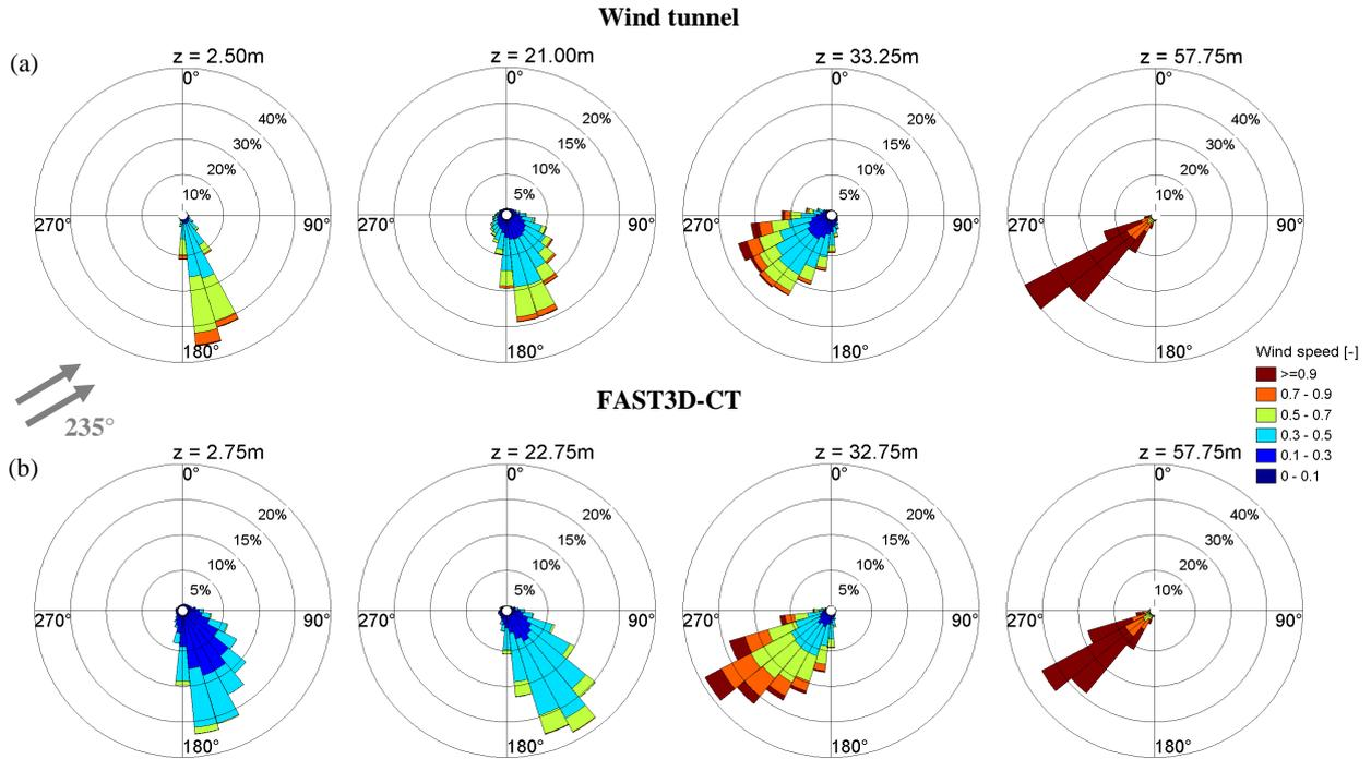
Figure 5. Wind-rose diagrams showing frequency distributions of horizontal wind speeds and wind directions for wind-tunnel measurements (a) and FAST3D-CT simulations (b) at four different heights within and above a street canyon (same location as in Figure 4a). Arrows on the left indicate the inflow direction.
