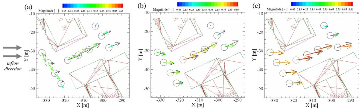
Figure 3. Mean horizontal velocity vectors of flow entering a courtyard at heights of (a) 3.5m, (b) 17m, and (c) 30m. Gray vectors represent wind-tunnel measurements. Color-coded vectors are from the numerical simulation with FAST3D-CT.
