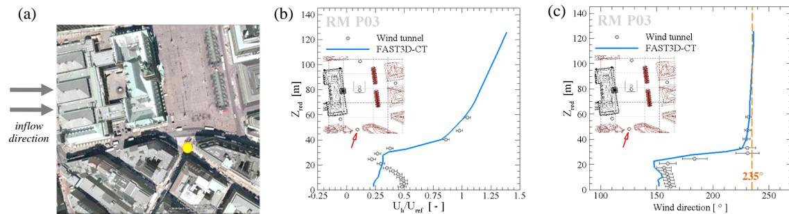
Figure 4. (a) Profile measurement location at a complex intersection; image extracted from Google Earth. (b) Mean horizontal wind speed and (c) wind direction profiles from wind-tunnel measurements and FAST3D-CT calculations.
