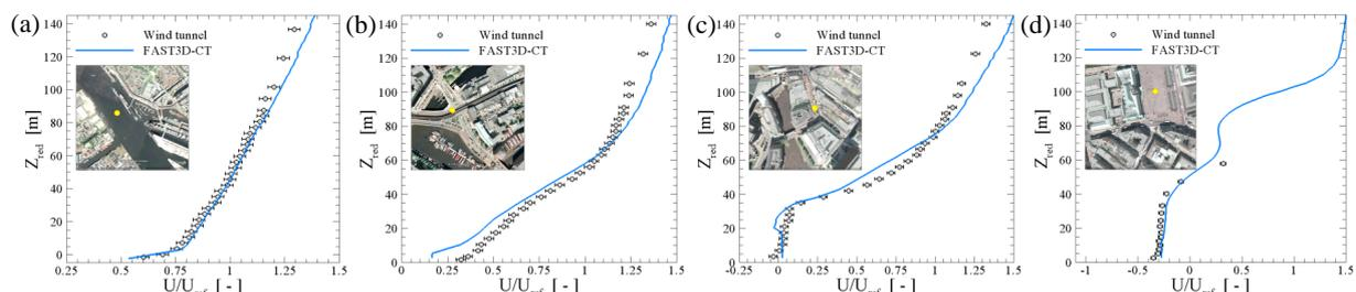
Figure 2. (a)-(d) Comparison of mean streamwise velocity profiles at various locations. Area images extracted from Google Earth.
