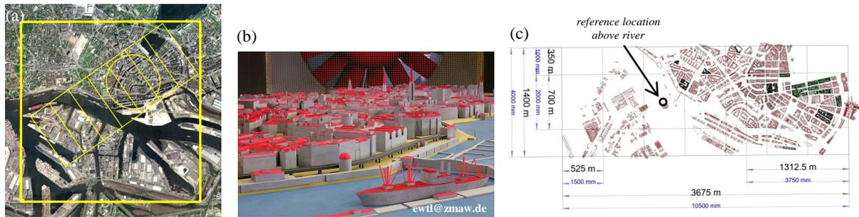
Figure 1. (a) Google Earth image showing the wind-tunnel model domain (inner frame) and the simulation region for FAST3D-CT (outer frame) of the inner city part of Hamburg. (b) Photograph of the urban wind-tunnel model. (c) Wind-tunnel model area with an indication of the reference location (framed dot) above the river.
