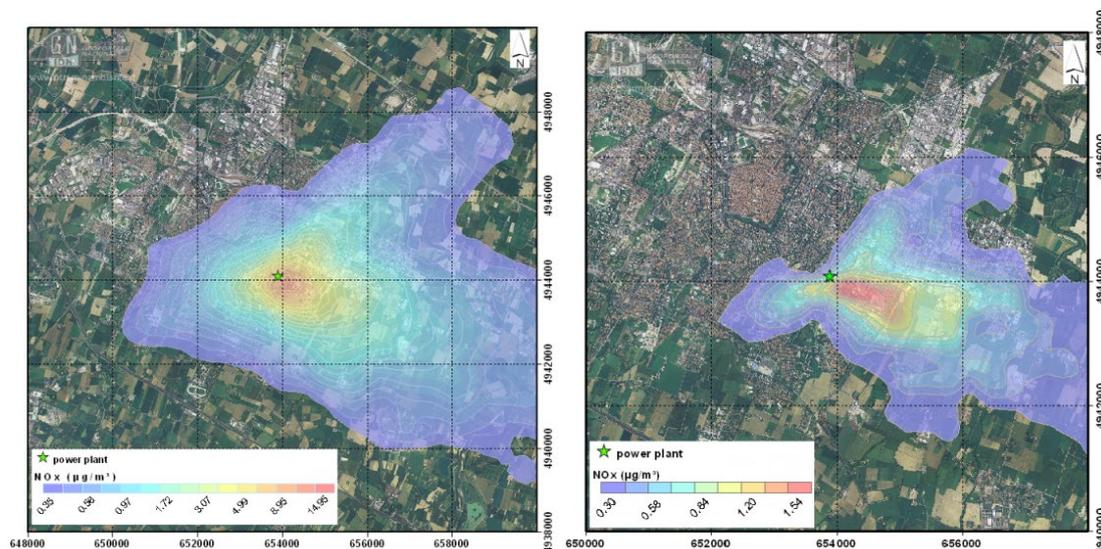
Figure 1. NO<sub>x</sub> concentration plumes at ground from the current Central Heating plant of the main hospital of Modena (left), and from the tri-generation plant (right), simulated by SPRAY. Simulation period ranges from January 1<sup>st</sup> to March 20<sup>th</sup> 2010. The plant stack location is the same both in the current and in the future scenario (the center point of the domain).
