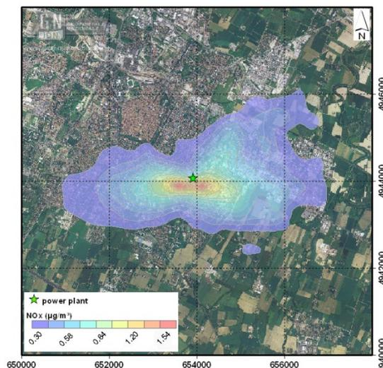
Figure 2. Annual average (year 2010)  $\text{NO}_x$  concentration plumes at ground from the tri-generation plant, simulated by SPRAY. The plant stack location is in the center point of the domain.
