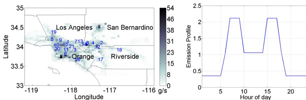
Figure 1. Gridded  $\text{NO}_x$  emissions and monitoring stations located in the South Coast Air Basin, Los Angeles. The right panel shows the assumed temporal profile of  $\text{NO}_x$  emissions.
