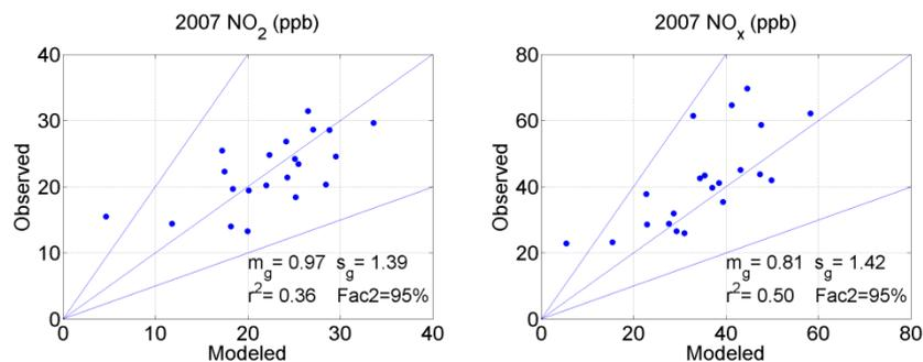
Figure 4. Comparison of modeled and measured annually averaged  $\text{NO}_2$  and  $\text{NO}_x$  concentrations at 21 sites in the SoCAB.
