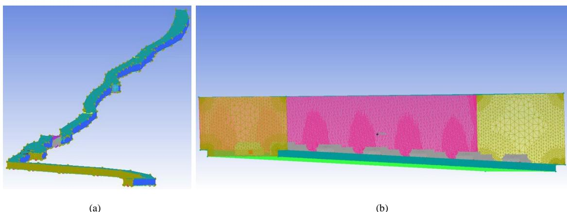
Figure 2. Tunnel geometry and mesh for (a) the entire segment from Basilica to Midi and (b) the field trial test section with vehicles
