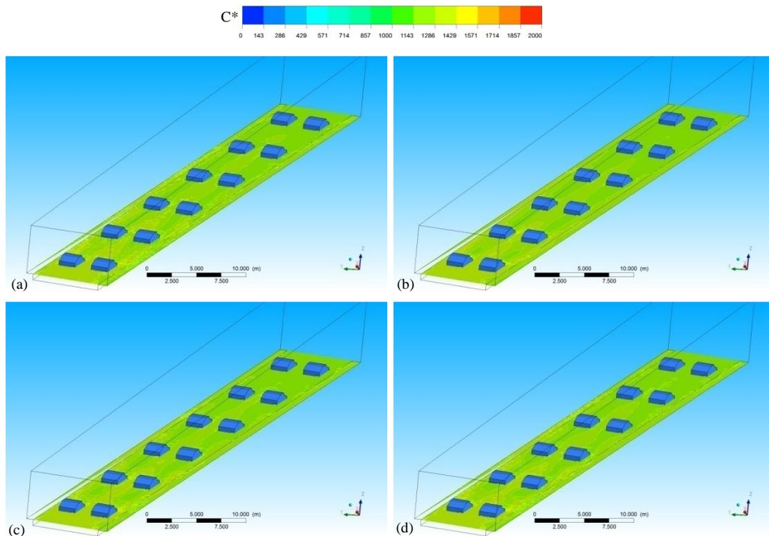
Figure 6. Non-dimensional concentration distribution along the field trial test section in the presence of moving vehicles at half the height of the vehicles at T = 5 s, T = 10 s, T = 15 s and T = 20 s
