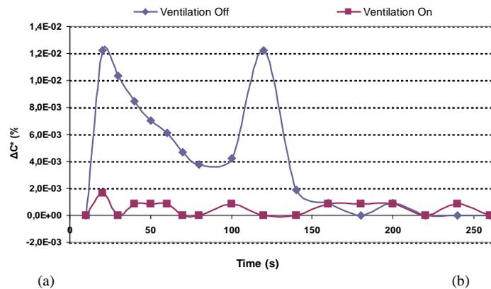
Figure 3. Non-dimensional concentration fluctuation in the direction Basilica – Midi over a period of 260 s
