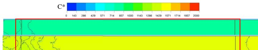
Figure 4. Non-dimensional concentration distribution along the field trial test section (shown in red) for the reference scenario on top and the ventilation scenario on bottom
