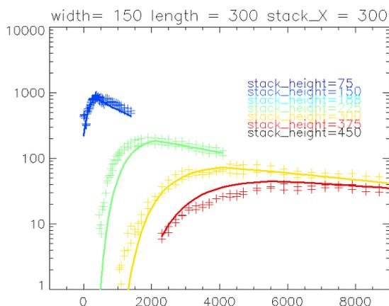
Fig.5: The reproduces GLC-profiles often fit nicely between GLC-profiles that have been measured twice, indicating that noise-fitting has been avoided by fitting curves through the optimal values for the parameters  $H_{final}$ . Displacement,  $B_f$  and  $A_f$ . +s denote the measurements, the lines show the model results.
