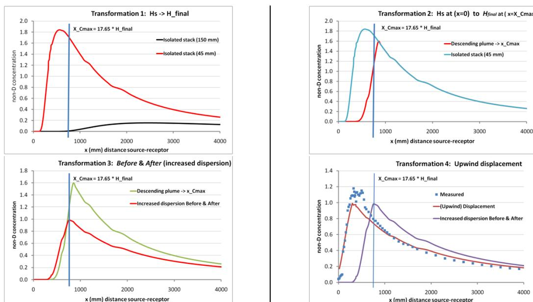
Fig. 4: Reproduction of a measured GLC-profile (Cubic building,  $H_s = H_b$ ,  $X_s = 2H_b$ ,  $H_b=150\text{mm}$ ) with  $H_{final}=45\text{mm}$ , Before = 434 mm, After = 175 mm and Displacement = -428 mm.
