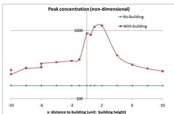
Fig.2 Peak values of measured GLC-profiles versus the position of stack to building for the cubic building,  $H_s=H_b$ .
