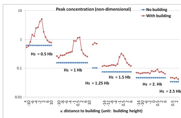
Fig.3 Peak values of GLC-profiles versus distance of stack to building for all the measurements with cubic building
