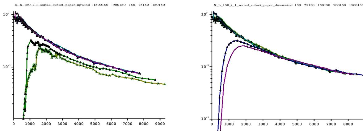
Fig. 1: Measured GLC-profiles for emissions through stacks of equal height  $H_b$  located on respectively the top of a cubic building (common curves on both graphs) and at positions  $X_s$  equal to  $10 H_b$  and  $6 H_b$  upwind (left) and downwind (right) of the upwind side of a cubic building.
