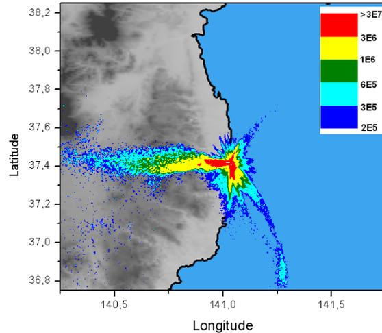
Figure 6. ARTM result of total Cs-137 and Cs-134 ground deposition in Bqm<sup>-2</sup> with DWD single point input near the site, without precipitation
