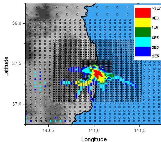
Figure 4. RODOS result of total Cs-137 and Cs-134 ground deposition in Bqm<sup>-2</sup> with TEPCO single point input at the site
