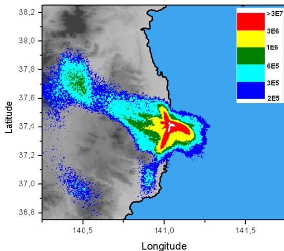
Figure 3. ARTM result of total Cs-137 and Cs-134 ground deposition in Bqm<sup>-2</sup> with TEPCO single point input at the site
