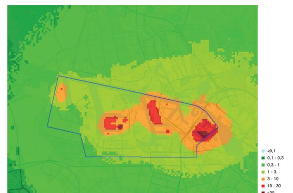
Figure 4. Calculated annual mean PM<sub>10</sub> concentrations due to emissions from the port region for 2009 (µg·m<sup>-3</sup>). The port region is indicated by the blue line.
