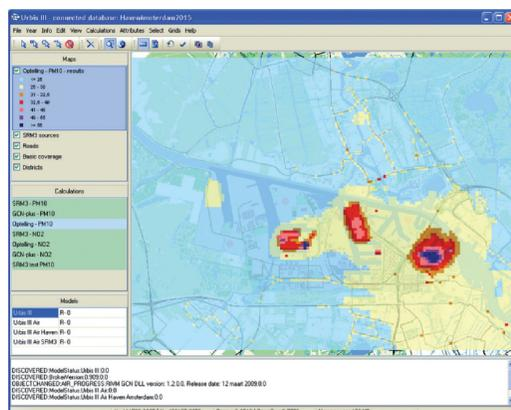
Figure 2. User interface of the air quality tool.
