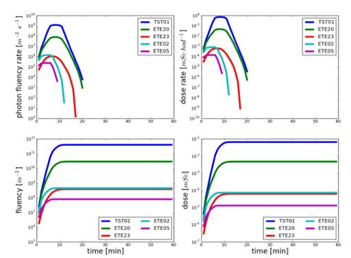
Figure 6: Time evolution of sensor response during spreading of smaller plume of 6 min duration of continuous  $^{131}I$  release.
