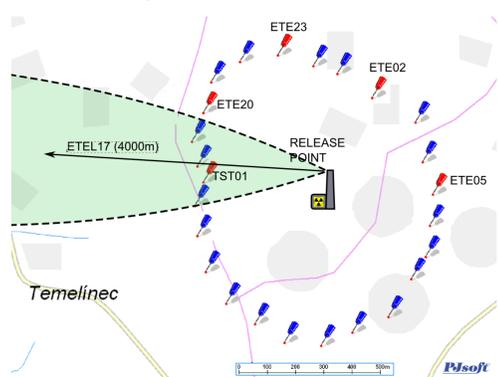
Figure 5: Tele-dosimetry ring on fence of NPP Temelin (24 detectors)
