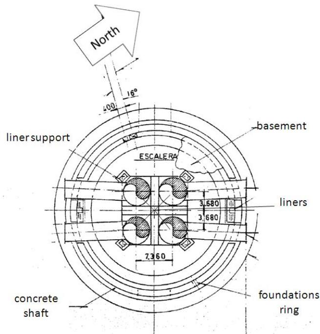
Figure 1. As Pontes Power Plant stack top view, with the four liners inside it. Measurements in mm and degrees (°).
