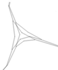
Figure 1. Roads were introduced as area sources in CALPUFF. As an example there is the motorway intersection in the south-western part of Ljubljana city.
