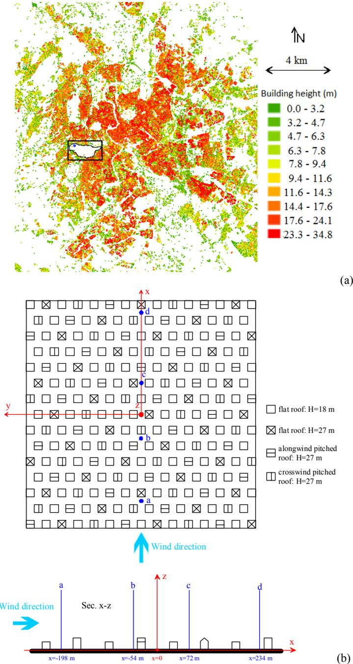
Figure 1. Rome area. Colors are building heights. The black line indicates VP park, the blue circle the position of the site. (b) CEDVAL experimental apparatus. The profiles a-d are those used for the analysis.
