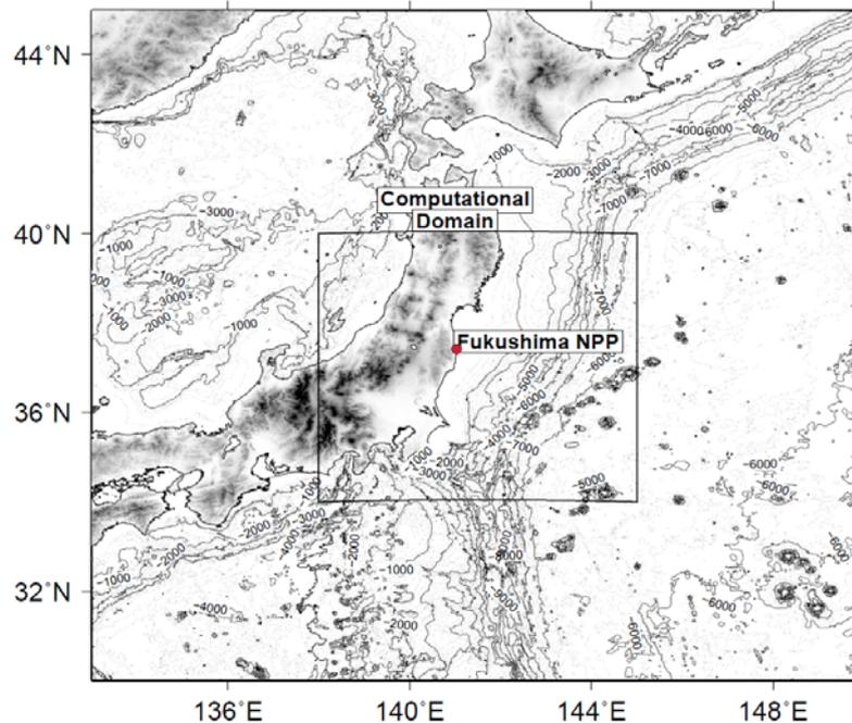
Figure 1. Computational domains for the numerical simulation of the concentration of  $^{137}\text{Cs}$  on seabed sediment
