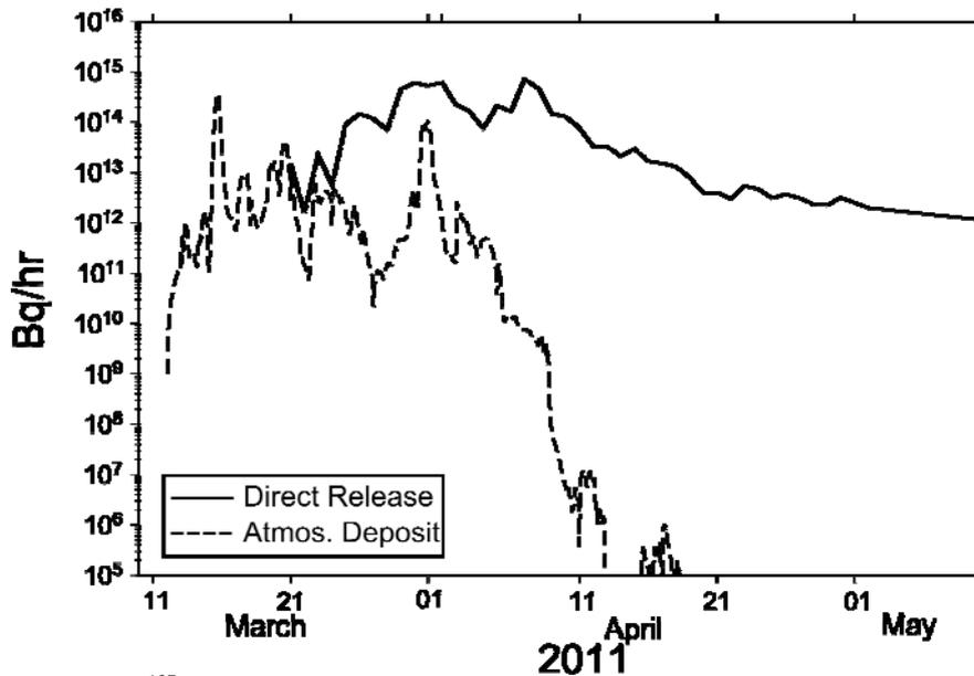
Fig. 3. Release rates of  $^{137}\text{Cs}$  due to direct release and atmospheric deposition.
