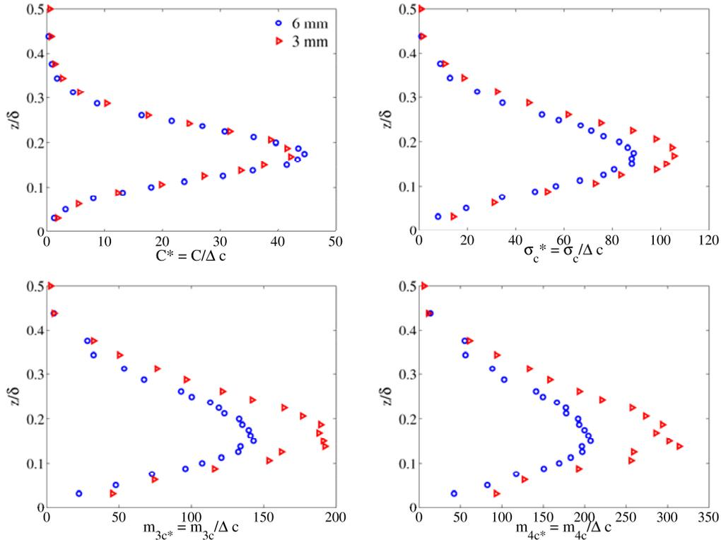
Figure 4. Vertical profiles of concentration statistics (mean, standard deviation, third and fourth moments) measured on the plume axis, at a distance  $x/\delta = 1.25$  from the emission point. Comparison between two source dimensions.
