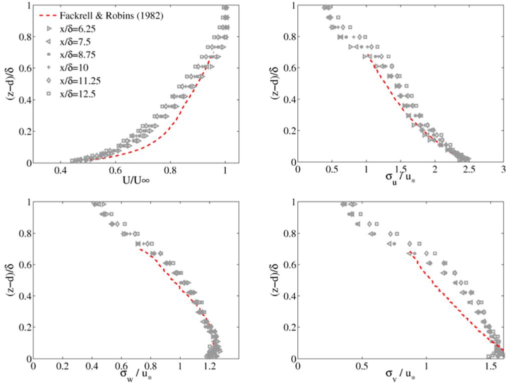
Figure 1. Normalised velocity profiles (mean  $U$ ,  $\sigma_u$ ,  $\sigma_w$ ,  $\sigma_v$ ) and comparison with literature data from Fackrell J. E. and Robins A. G., 1982b.
