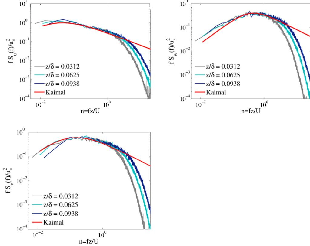
Figure 2. Velocity spectra for growing distances from the wall  $z/\delta$  for the three velocity components. Comparison with model extrapolated from field data (Kaimal et al., 1972).
