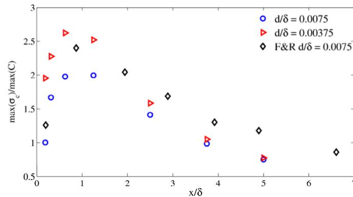
Figure 6. Development of the intensity of concentration fluctuations  $\max(\sigma_c)/\max(C)$ , at every downstream position. Comparison with Fackrell J. E. and Robins A. G. (1982b).
