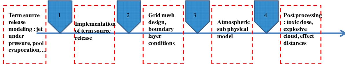
Figure 1 : Main calculation stages to simulate atmospheric dispersion of an accidental release (toxic or flammable gas release)
