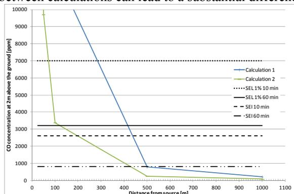
Figure 2 : calculated concentration of CO at 50 m, 100 m, 500 m for two calculations of the first test case ; SEI 10 min stands for *Seuil effet irréversible* is the threshold of irreversible effects for 10 min exposure; SEL 1% stands for *Seuil effet léthal* is the threshold of first lethal effects above which 1% mortality can be observed in the exposed population
