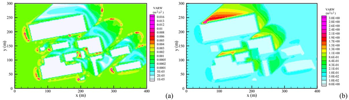
Figure 3. Horizontal section of the vertical velocity variance calculated by micro-SWIFT at (a)  $z=1$  m and (b)  $z=10$  m.
