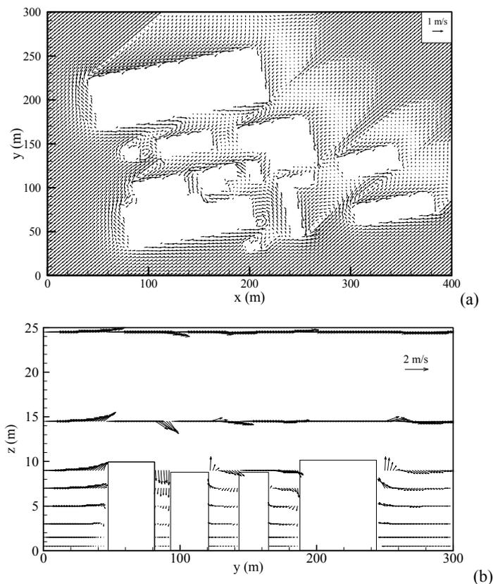
Figure 2. (a) Plane view of the velocity vectors calculated by micro-SWIFT at  $z=10$  m. (b) As in (a), but for the vertical section at  $x=160$  m.
