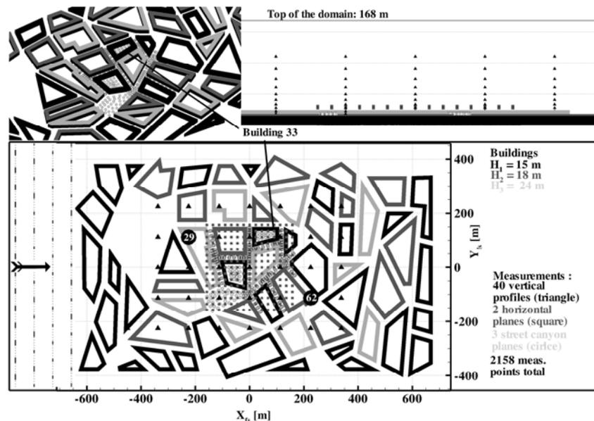
Figure 1. Building layout, computational domain height and measurement positions for the test case Michel-Stadt
