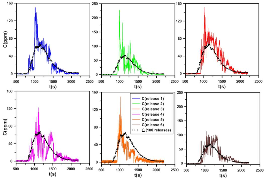
**Fig.1.** Comparison between the concentration measurements for six different realizations and the average concentration (dashed line) over 100 realizations in receptor located at coordinates (X= 1200m, Y=0, Z= 24m, X being the wind direction).
