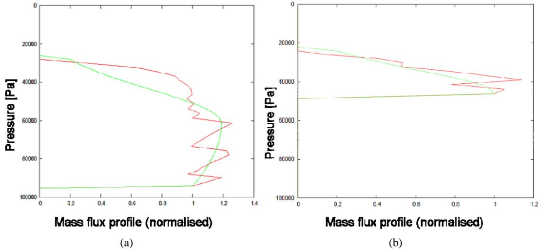
Figure 3. The figure shows the mass flux profiles obtained with (a) equation (4) and with (b) equation (5) (green dashed line) compared with those provided by the SCM (red solid line), for two given times.
