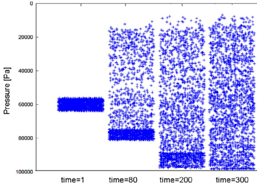
Figure 2. Time snapshots of particle distribution in the environment column. Time shown is the number of time steps.
