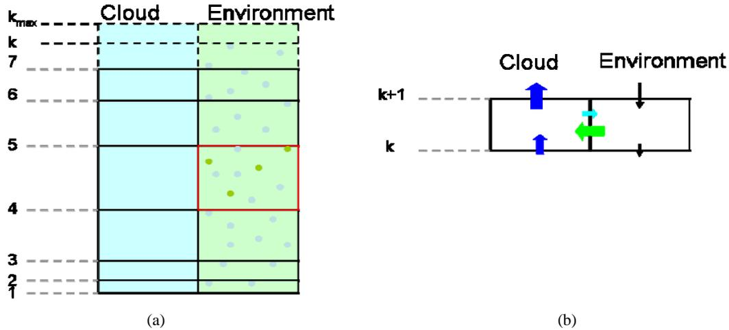
Figure 1. (a) represents the environment and the cloud columns used in the model for vertical transport. The particles that entrain between level 4 and 5 are shown in green. (b) shows a sketch of updraught mass fluxes (blue arrows) and the entrainment and detrainment fluxes (respectively green and sky-blue arrows) between two pressure levels.
