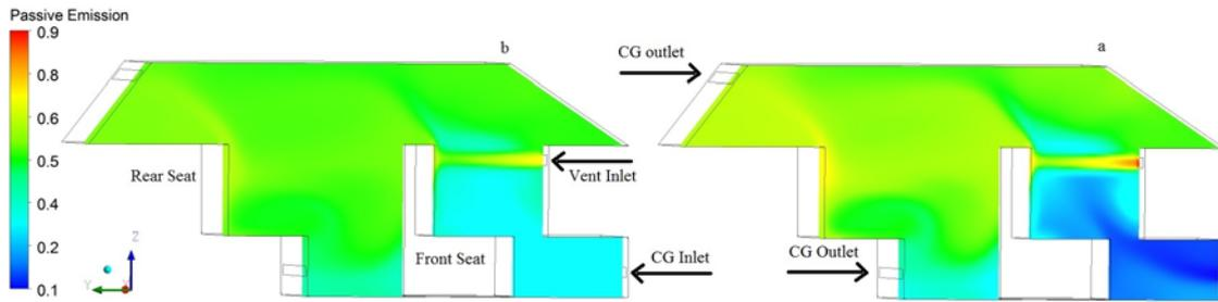
Fig. 1: Isotropic view of half of a simplified car cabin for two scenarios: (a) emission penetration into the cabin is mainly through ventilation system (Vent/CG = 90/10 %), and (b) emission is filtered in the ventilation system (Vent/CG = 70/30%). The outer boundary of the vehicle is removed and the cabin boundary is only visible.
