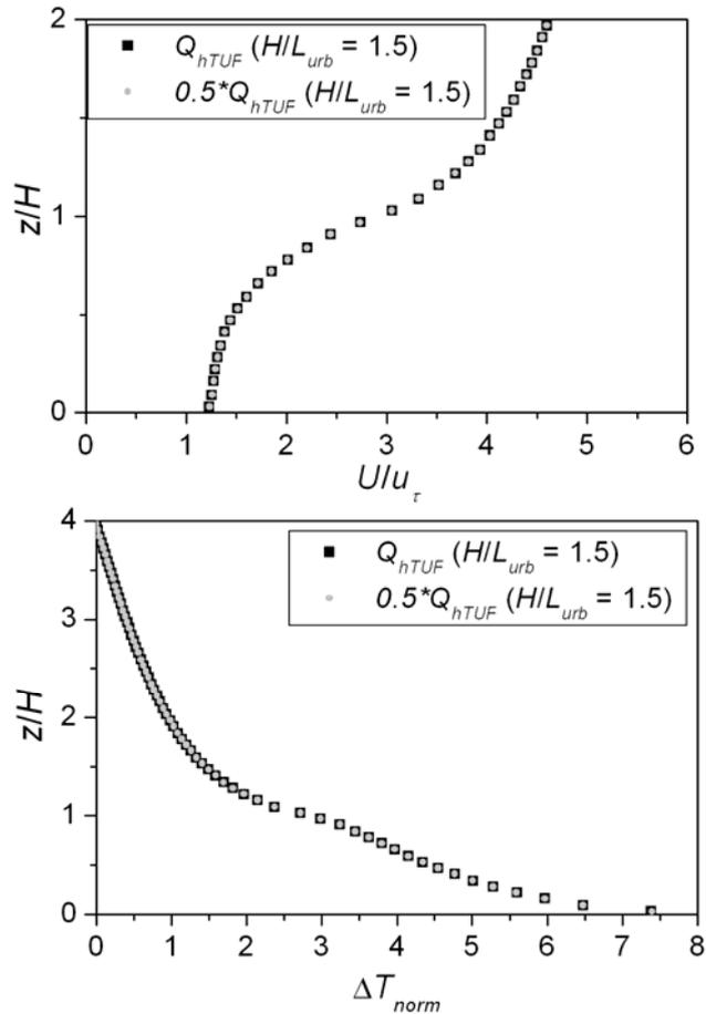
Figure 2. Vertical profiles of spatially-averaged streamwise velocity and  $\Delta T_{norm}$  for cases with the same  $Q_{hnorm}$  ( $= 1.5$ )
