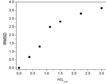
Figure 4. RMSD comparing average streamwise velocity vertical profiles of cases with different  $H/L_{urb}$  with the neutral case ( $Q_h = 0$ ). Values are compared from  $z/H = 0$  to  $z/H = 2$ .
