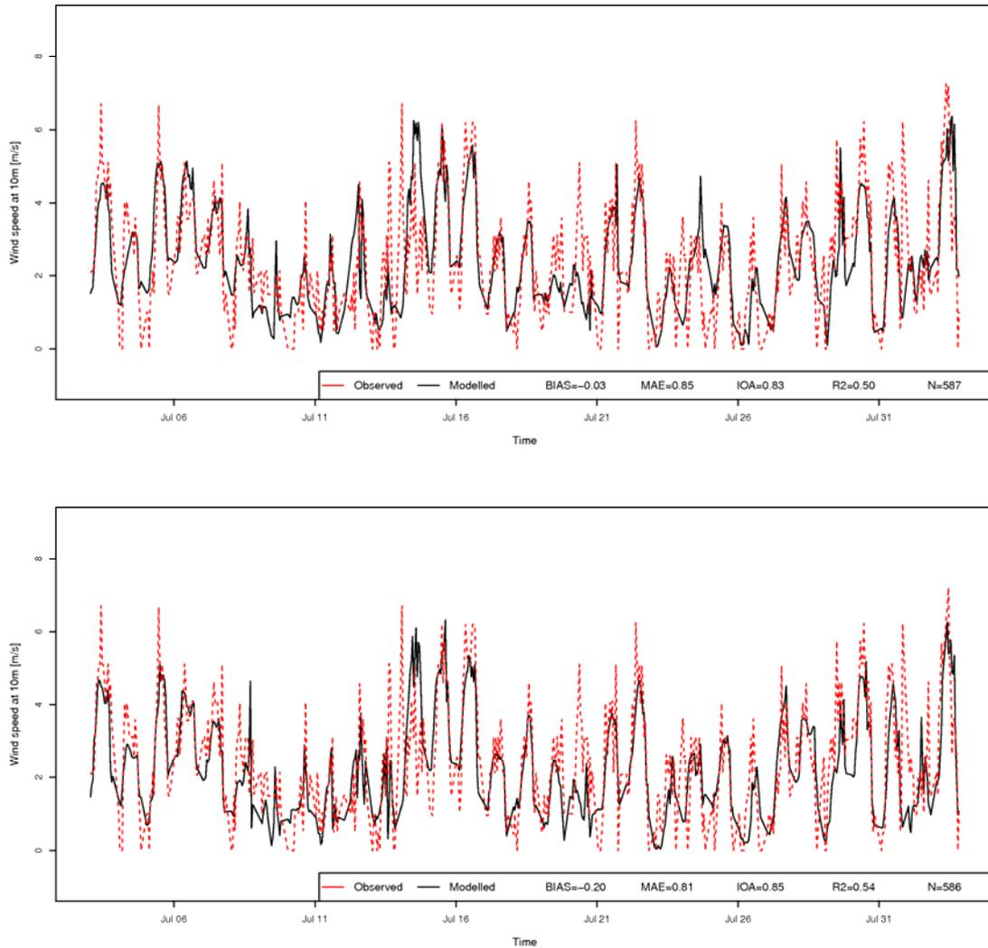
Figure 3. Modelled vs. measured wind speed in Wrocław: ERA-Interim (top) and NCEP FNL (bottom).
