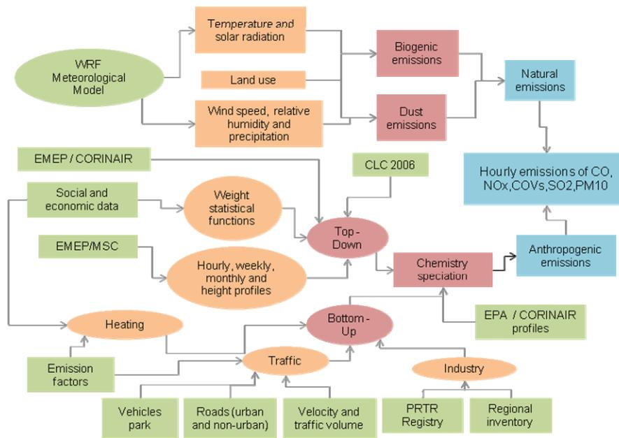
Figure 2. Air Emission Model Scheme.
