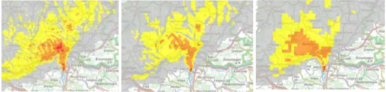
Figure 1: External cloud dose prognosis map overlays for three different horizontal spatial grid resolutions. From left to right: 250 m, 500 m, and 1'000 m; time resolution 10 min and high statistics number of particles for scenario F. Maps courtesy of SwissTopo.
