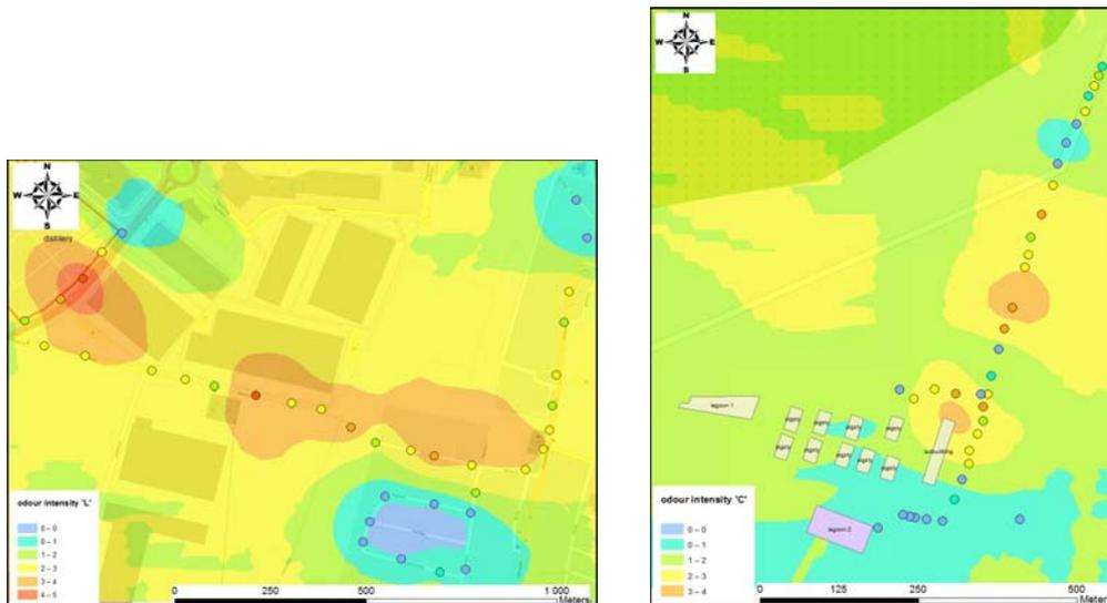
Figure 2. Odour intensity spatial distribution obtained by geostatistical interpolation, using Ordinary Kriging method A) for a measurement shown on figure 1A (distillery), B) for a measurement shown on figure 1B (swine farm).
