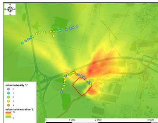
Figure 3. Odour concentrations spatial distribution ( $ou_E/m^3$ ) obtained by calculations using CALPUFF model, during 4th series of field measurements.
