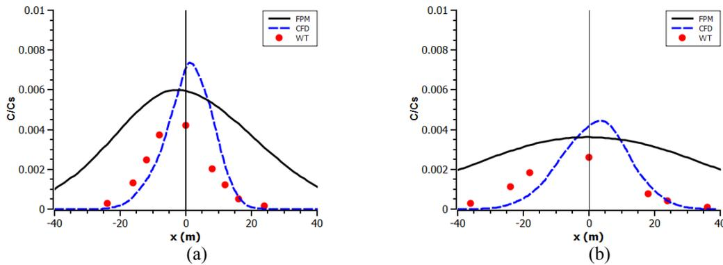
Figure 3: (a) non-dimensional average lateral concentration levels ( $x=50$  m,  $z=1.6$  m); (b) non-dimensional average lateral concentration levels ( $x=100$  m,  $z=1.6$  m).
