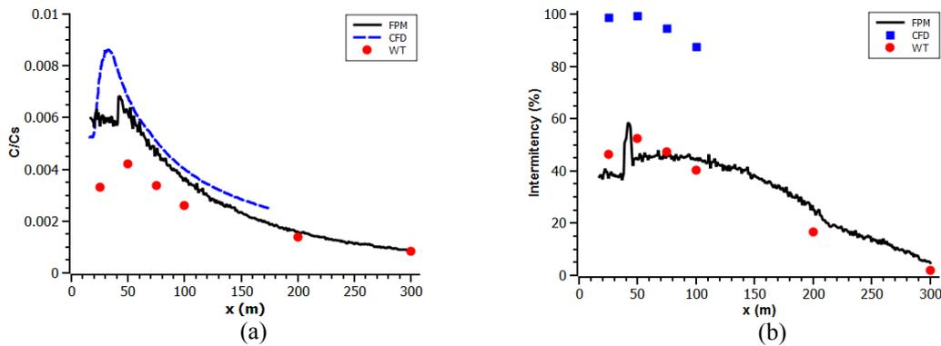
Figure 2: (a) non-dimensional average downwind concentration levels ( $z=1.6$  m); (b) downwind intermittency levels ( $z=1.6$  m).
