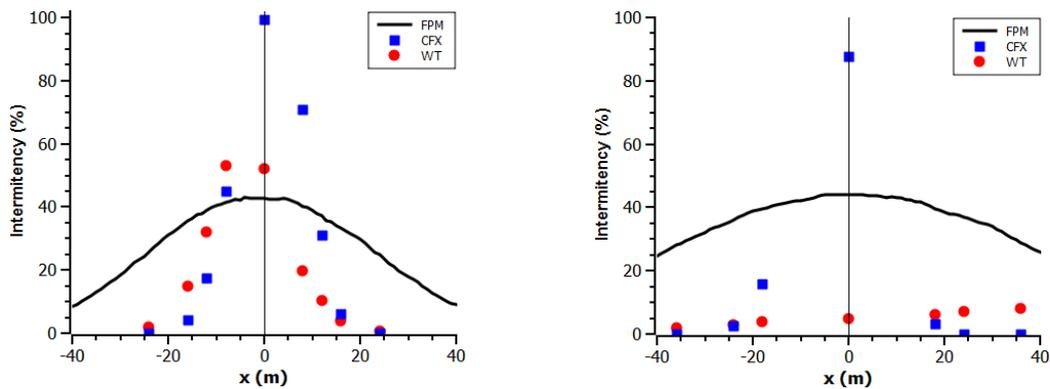
Figure 4: (a) lateral intermittency levels ( $x=50$  m,  $z=1.6$  m); (b) lateral intermittency levels ( $x=100$  m,  $z=1.6$  m).
