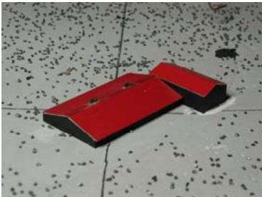
Figure 1: model of the obstacle used in the wind tunnel experiments (CEDVAL, 2002)
