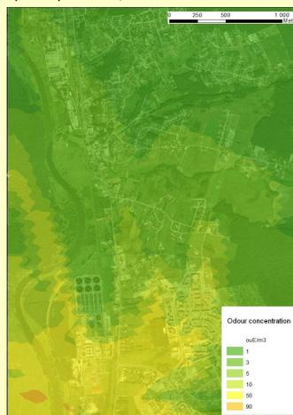
Fig. 8. Maximum odour concentration - thermal drying plant, summer season
