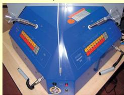
Fig. 4. Dynamic olfactometer TO8
