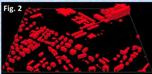
Fig. 2: Building geometry, deduced in a GIS from a high-resolution 3D cartography.
