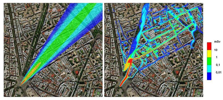
Total Effective Dose Equivalent (in mSv) resulting from the atmospheric dispersion of a radiological threat agent (3 TBq of <sup>137</sup>Cs) as seen by a simple Gaussian model and by a Lagrangian Particle Dispersion Model taking the buildings into account
