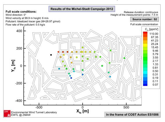
✓ Data gathered during a wind-tunnel flow and dispersion experiment (Hamburg University) – several continuous/puff releases in different locations; open and blind tests ✓ A typical European urban site is reproduced, designed to include potential inhomogeneities, characterising the neighbourhood-scale urban areas across Europe
