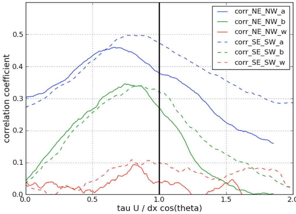
Spatial cross-correlation of anemometers (NE,NW) and (SE,SW) as a function of a normalized time lag
