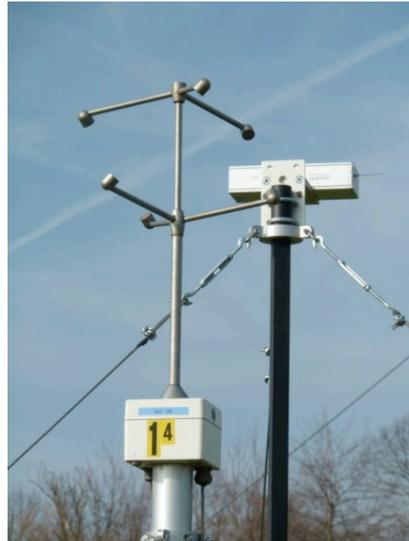
Ultrasonic anemometers (front)
