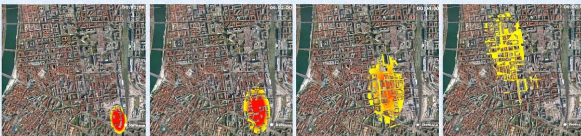
Fig. 2. Instantaneous activity concentration 1, 2, 4, and 8 minutes after a fictitious explosion in “La Part-Dieu” railway station in Lyons.
