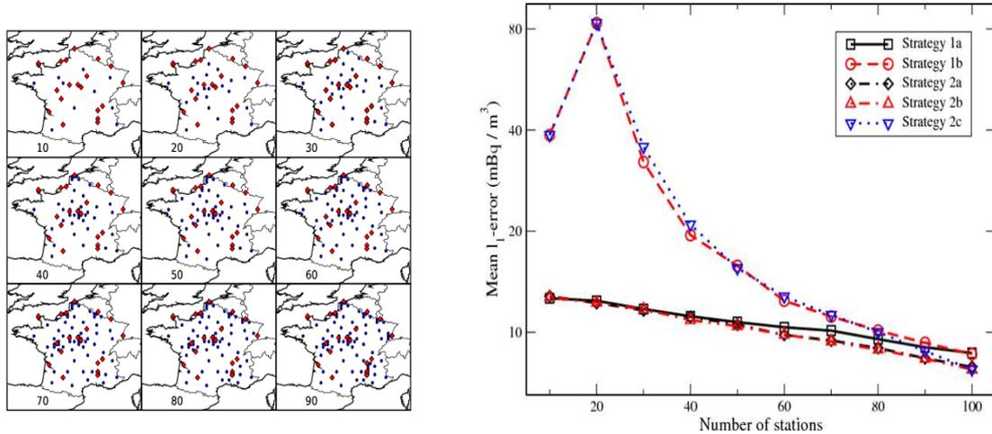
Figure 2. Sequential deployment of the network following strategy 2b (left). The red rhombuses are the nuclear sites. The blue disks are the optimised monitoring stations. Mean error for deployment strategies (right)
