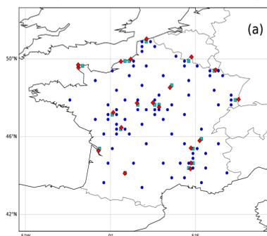
Figure 1. Reference optimal network for 100 stations. The red rhombuses are the nuclear sites. The green squares stand for the fixed stations. The blue disks are the optimised monitoring stations.
