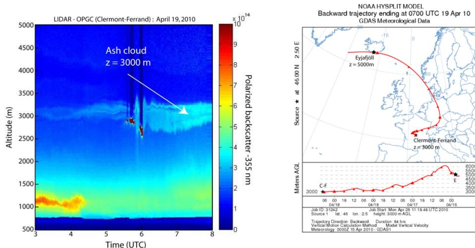
Figure 5. Lidar ash cloud detection. The ground-based Lidar-OPGC located at Clermont-Ferrand, has permitted the very accurate detection of ash above Clermont-Ferrand (France), at an altitude of 3000m, on April 19. The backward trajectory calculation carried out with NOAA-Hysplit model permits to validate and confirm source information such as the altitude and start date of the ash cloud emission at Eyjafjöll volcano.
