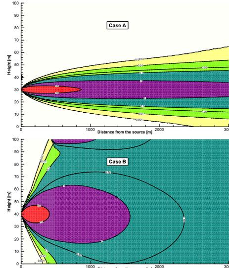
Figure 9: Case A and B for HPDM: plume longitudinal section.
