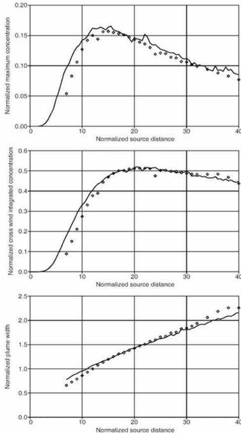
Fig.1 Comparison between results from wind tunnel (diamonds) and AUSTAL2000 (solid line)
