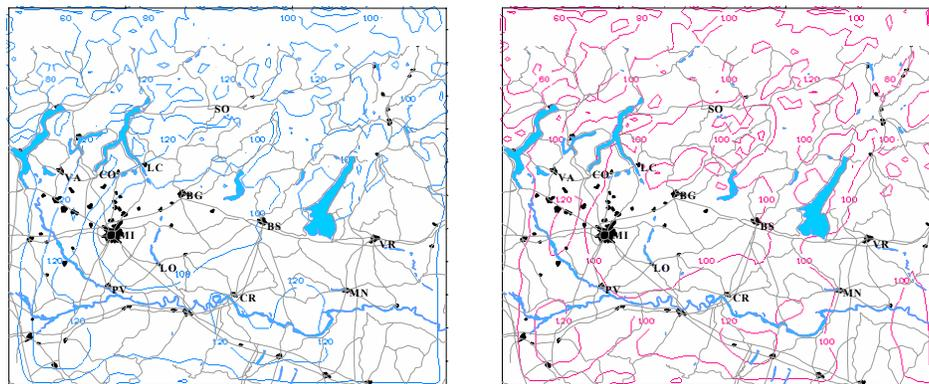
Figure 3. Ozone fields evaluated by the (a) SAPRC97 and (b) CB4 mechanism at 16 PM, June 4, 1998.
