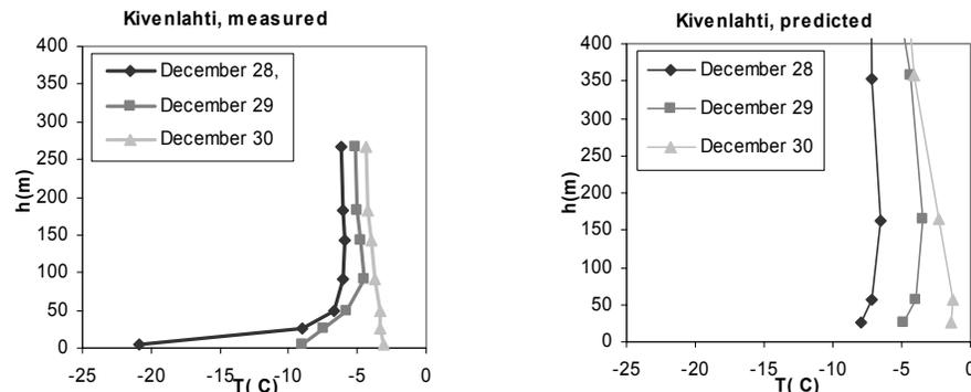
Figures 3a-b. The evolution of the measured (a) and predicted (b) temperature profiles at the Kivenlahti mast from 28 to 30 December, 1995 at 00 UTC (Universal Time Coordinated). The measurements were conducted at the radio tower of Kivenlahti, and the predictions were computed with the numerical weather prediction model HIRLAM, a version that was operational in 2001 (4.6.2).
