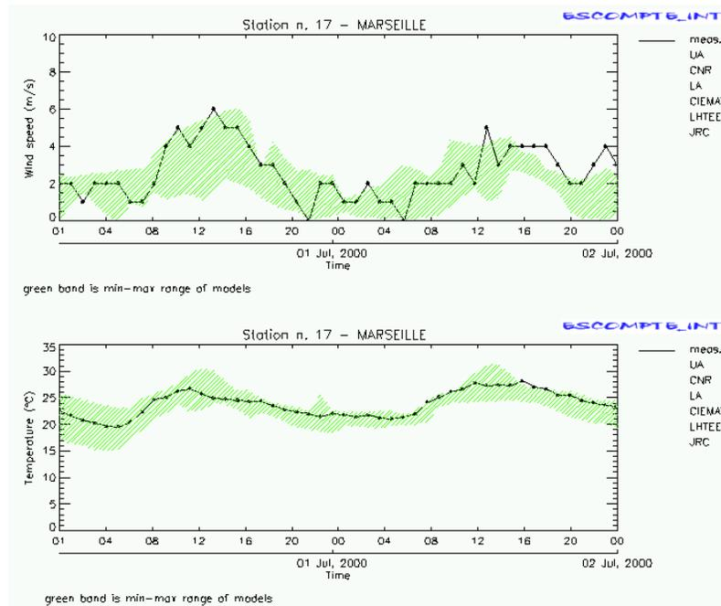
Figure 5. Range of wind speed and temperature in Marseille on 1 July 2000 resulting from simulations with six different urban scale models compared to corresponding results of the ESCOMPTE pre-campaign (cf. [http://rem.jrc.cec.eu.int/escomppte\\_int/RESULTS/](http://rem.jrc.cec.eu.int/escomppte_int/RESULTS/)).
