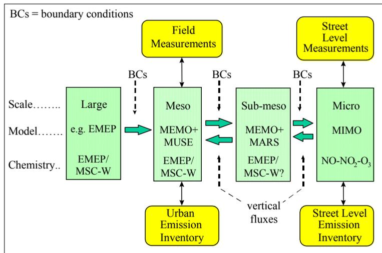
Figure 2. Schematic presentation of a multi-scale model cascade for evaluating urban air pollution levels (Moussiopoulos et al., 2000).
