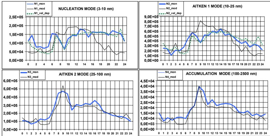
Figure 1. Particle number concentrations in Stockholm: Measured (thick line) vs. computed values (thin line: constant emission factors, dashed line: velocity dependent emission factors) for various modes. The results demonstrate the need for an emission factor correction in the case of the finer modes (Johansson, 2002).
