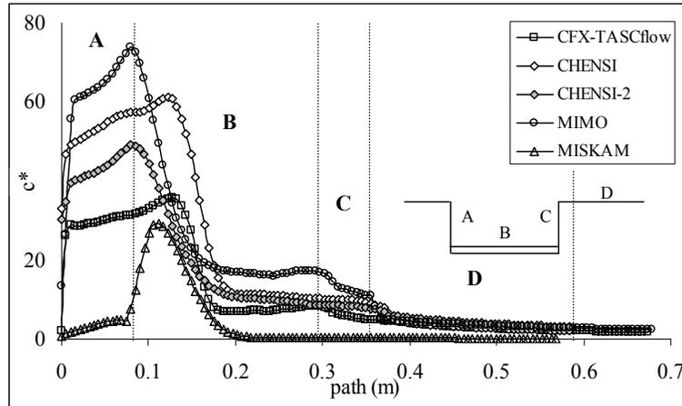
Figure 4. Comparison of the normalised concentration  $c^*$  along the path ABCD for the cavity with  $W/H=2$  (A and C correspond to 75% of the cavity depth, while B and D are equal to its width) after Sahn et al. (2001).
