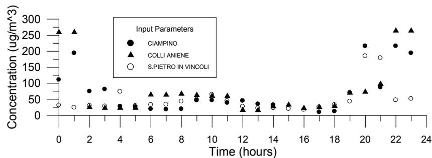
Figure 3. Comparisons among concentrations calculated by ADMS-Urban, making use of input wind data taken at different weather stations on 14 June 2002.
