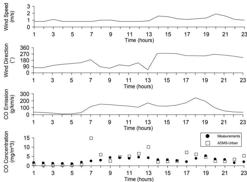
Figure 4. Comparison between measured and modelled CO concentrations on 27 November 2001. The corresponding wind and emission input data have been reported above.
