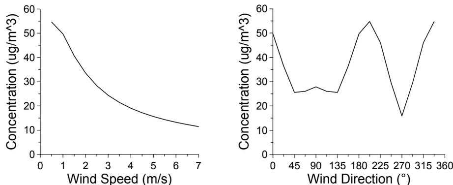
Figure 1. Pollutant concentration calculated by ADMS-Urban versus wind speed and wind direction, for a road source located in a street canyon.
