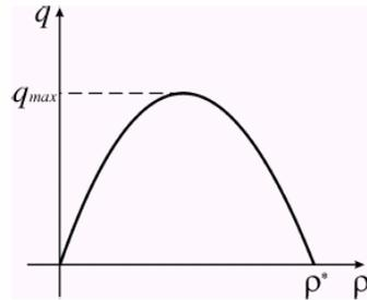
Figure 2. Fundamental traffic diagram.
