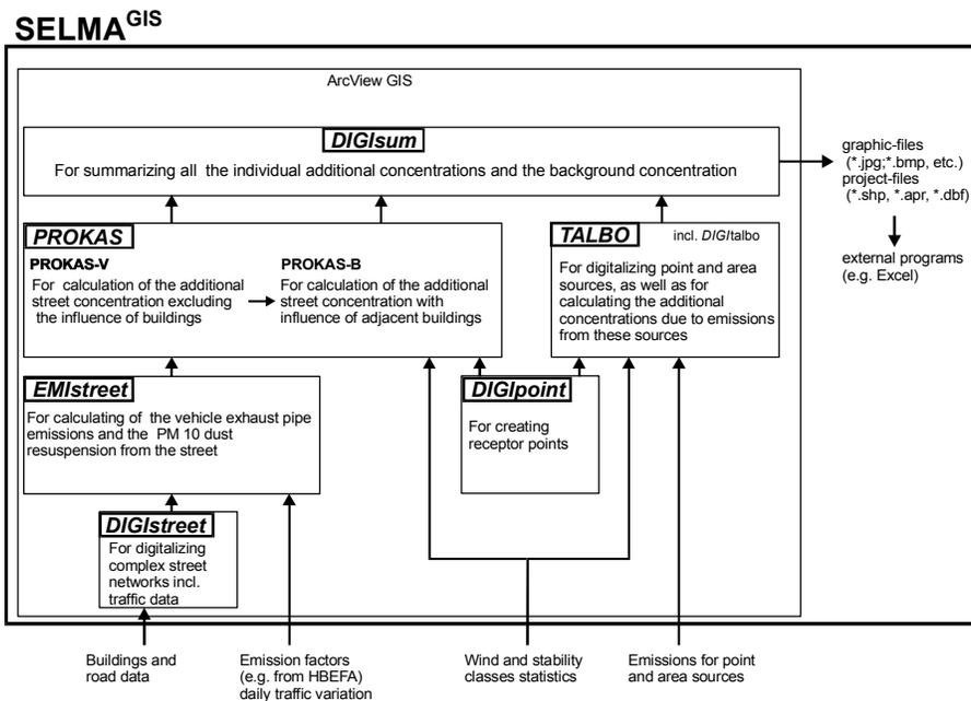
Figure 1. SELMA<sup>GIS</sup> Model Diagram.
