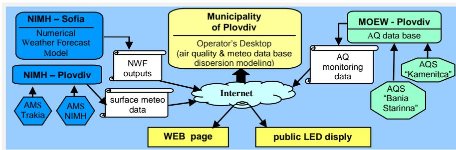
**Figure 1.** Structure and data flow diagram of the Plovdiv's AQMS. AQS - air quality station, AMS - automatic meteorological station, MOEW - Ministry of Environment and Waters
