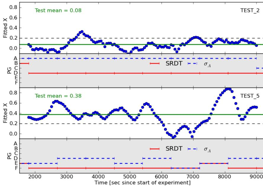
**Figure 4** Fitted exponent X (blue dots) and Pasquill-Gifford stability class (PG) over time for tests 2 (top) and 5 (bottom). The test's average fitted exponent is represented by the green line. The dotted black line shows the value used in ARTM.
