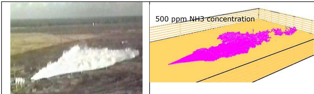
**Figure 5:** comparison between the overall form of the experimental cloud shape and simulation results
