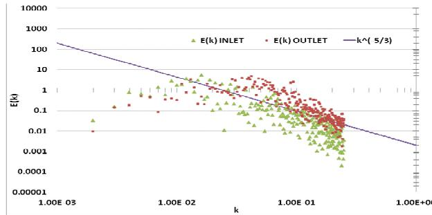
**Figure 4:** comparison of the turbulent energy spectrum at the inlet and outlet conditions
