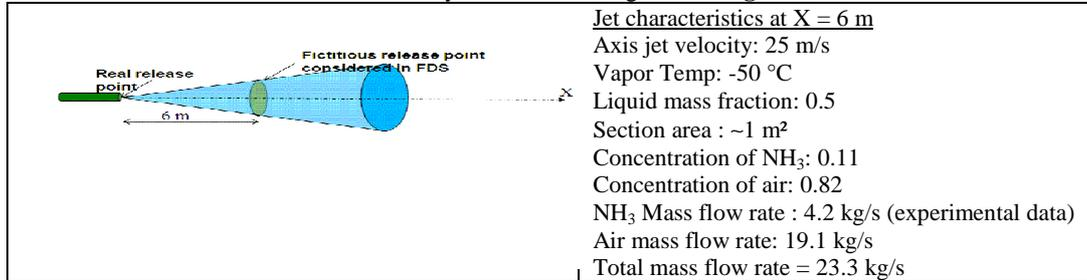
**Figure 2:** description of the term source implemented in FDS simulation
