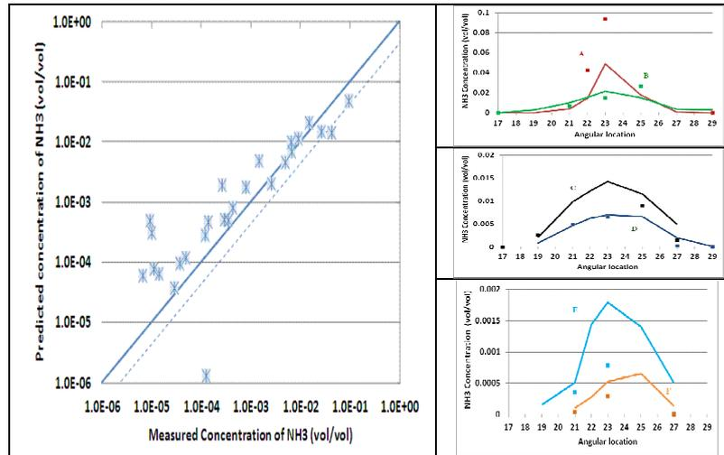
**Figure 6:** Comparison between simulation results and experimental data for the whole set of receptors (logarithm scale)(left graph) and for each arc (A, B, C, D, E,F) of receptors (right graphs)
