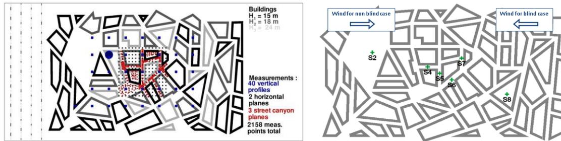
Figure 1. Computational domain with buildings, wind velocity measurement positions and sources positions.
