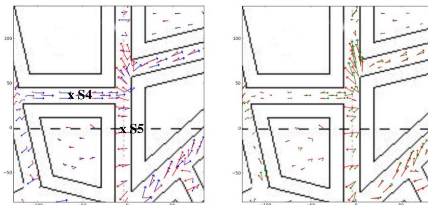
**Figure 5.** Wind field at a height of 7.5 m near sources S4 and S5 (PMSS in blue, Code\_SATURNE in green and observations in red).
