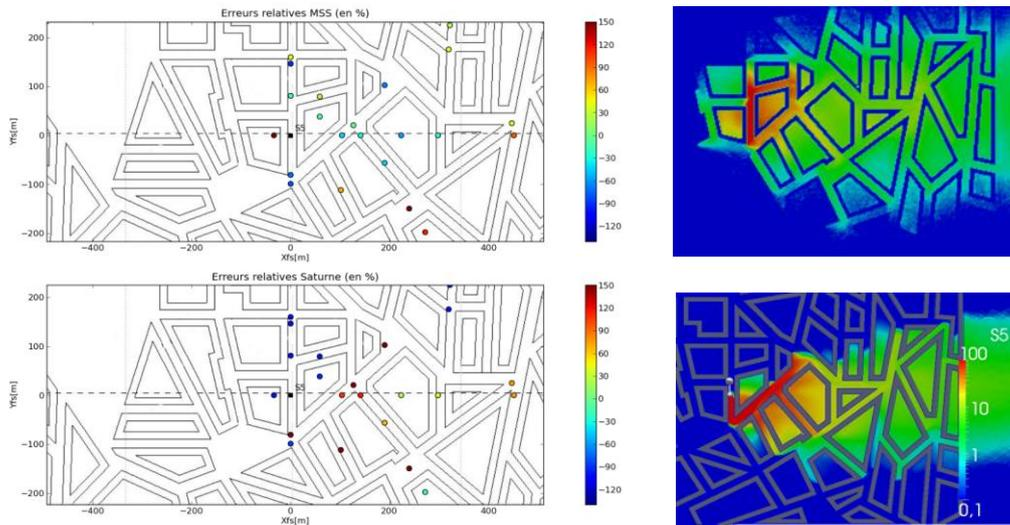
**Figure 4.** Concentration field at a height of 7.5 m and relative errors compared to observations for continuous release from source S5 (PMSS at the top and Code\_SATURNE at the bottom).
