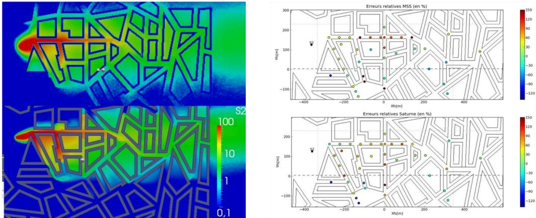
**Figure 2.** Concentration field at a height of 7.5 m and relative errors compared to observations for continuous release from source S2 (PMSS at the top and Code\_SATURNE at the bottom).
