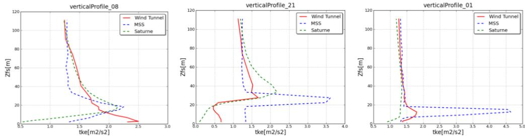
**Figure 3.** Vertical profiles of TKE upwind a building (left), inside a street canyon (middle) and downwind (right).
