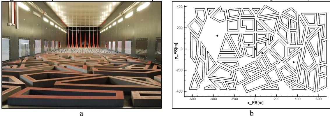
**Figure 1.** Model of Michelstadt in the wind tunnel (a). Layout of the model (b).
