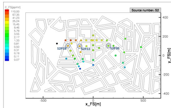
**Figure 2.** Results of the continuous release measurements from S2 source.
