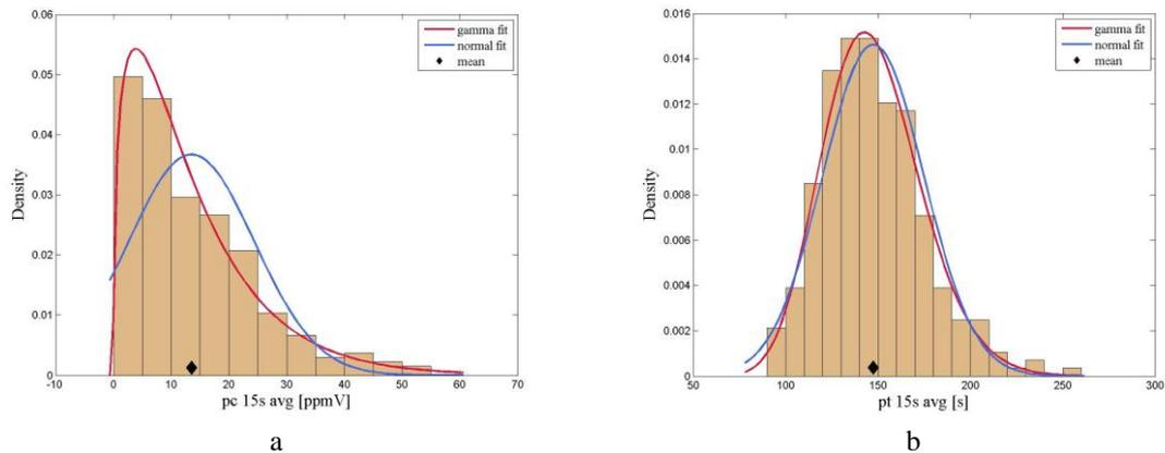
**Figure 4.** Probability density of the peak concentration (a) and peak time (b) of the 15-s-averaged puff release dispersion time series for measurement point S2P22.
