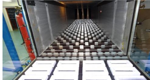
Figure 2. Development of the boundary layer in the tunnel.
