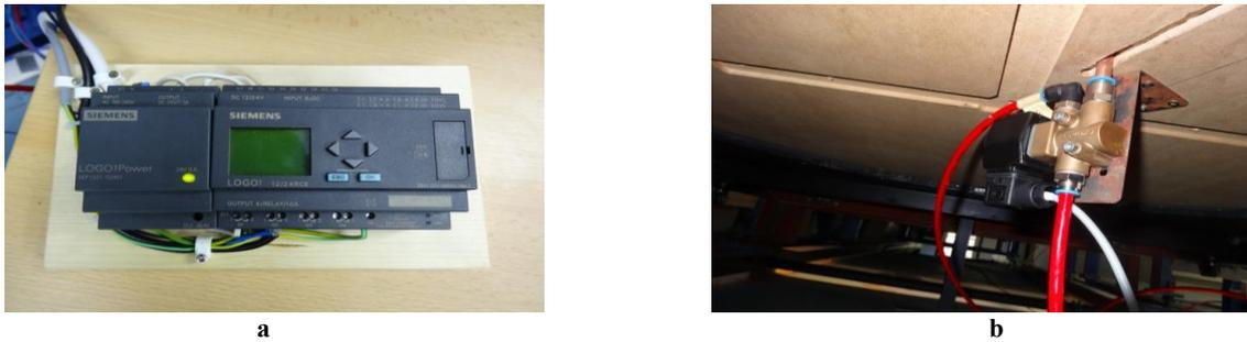
**Figure 4.** Equipment for puff creation – PLC Siemens LOGO! (a) and electromagnetic valve of Norgren (b).
