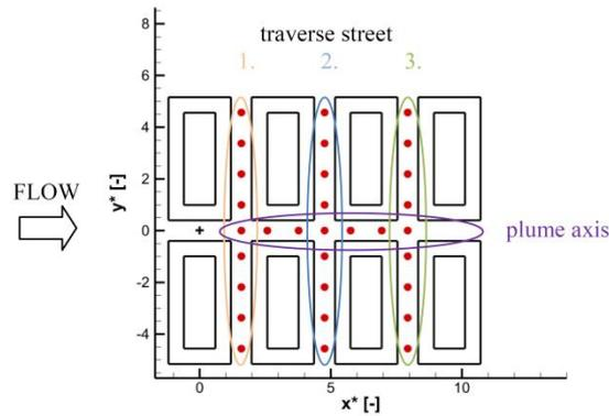
**Figure 6.** Scheme of investigated section (the source position is denoted as a black cross; red filled circles represent sampler places).
