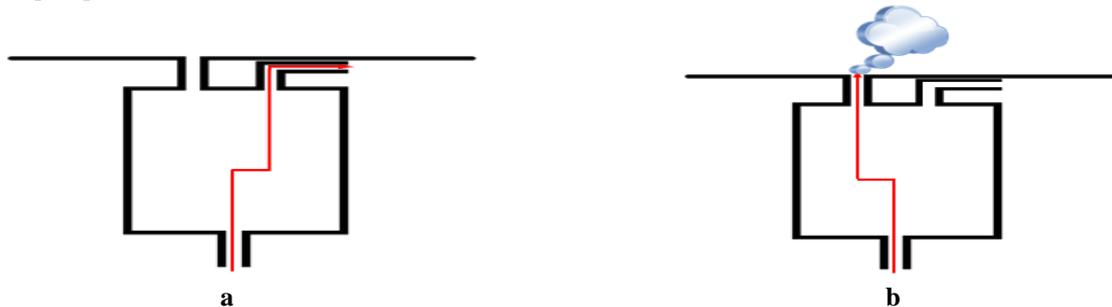
**Figure 5.** Principle of puff creation in the tunnel – valve without voltage (a) and under voltage (b).
