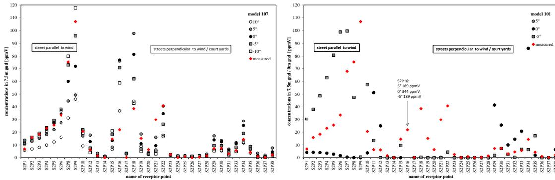
**Figure 2.** Comparison between measured and modelled average concentrations (left: model 107, right: model 101) for a continuous release from source S2 with variations in approach flow directions.
