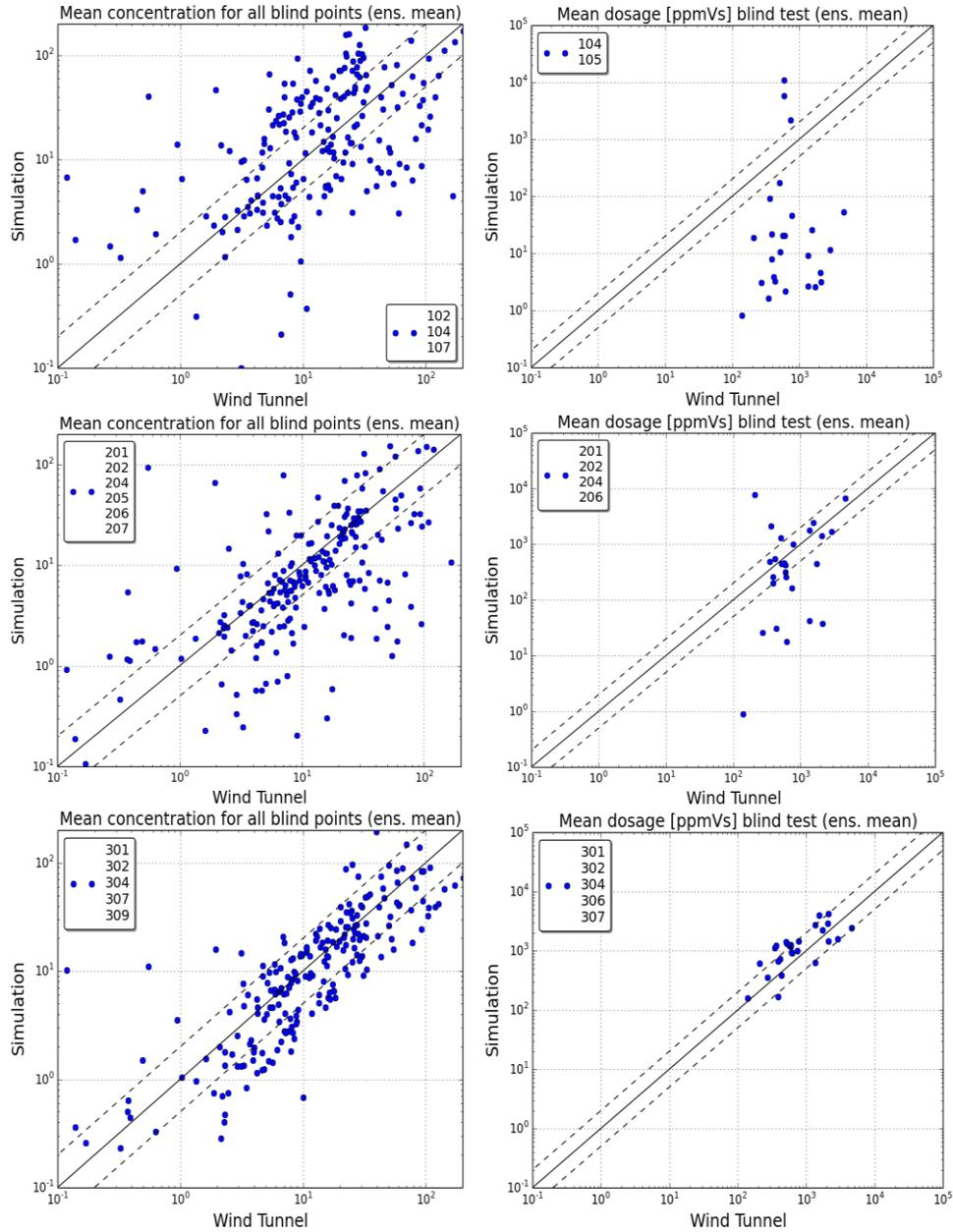
**Figure 3.** Measured versus ensemble averaged modelled mean concentrations (left) and dosages (right) at receptors for continuous releases (left) and puff releases (right) for model Type I (top left), II (top right) and III (bottom left).
